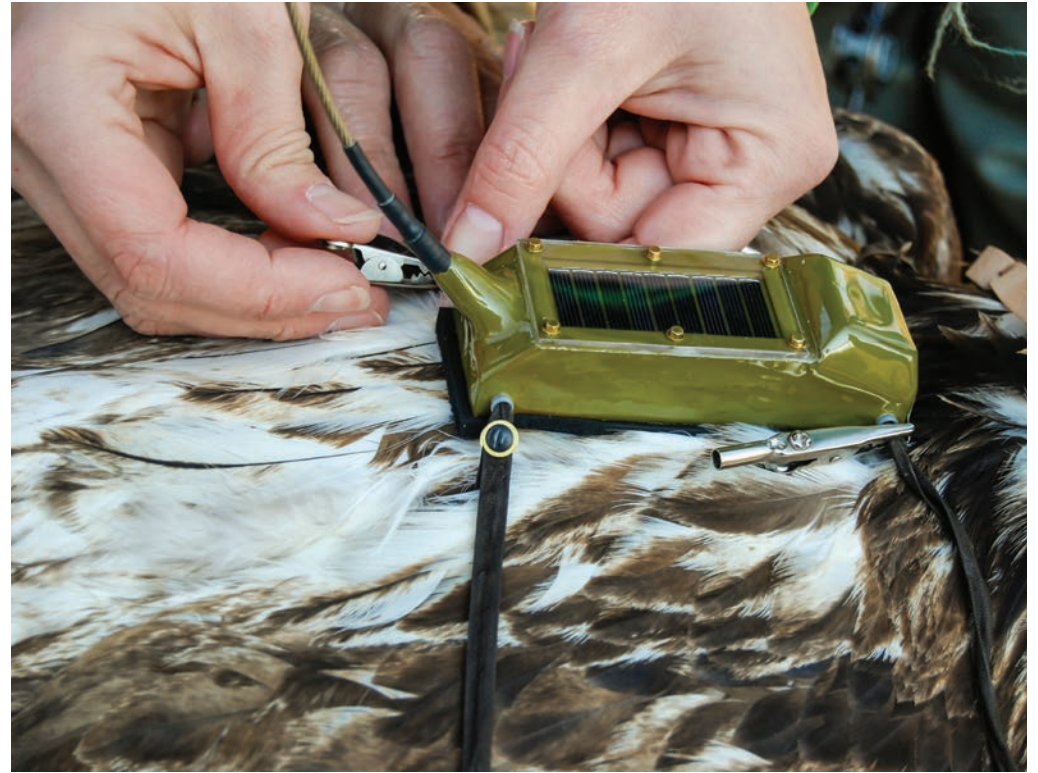
Libby Mojica attaches a transmitter to a second-year bald eagle. Tracking eagles with satellite transmitters has allowed The Center to effectively assess winter home ranges. Photo by Bryan Watts
